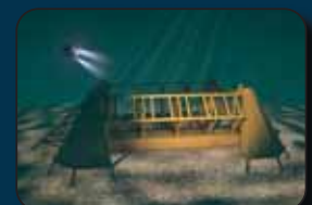
Landing template on seabed
